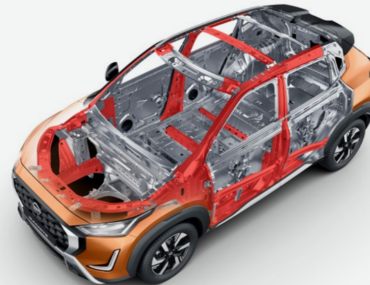
67% Usage Of High Tensile Strength Steel
